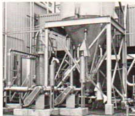
The 4" O.D. blending tubes are connected to the circumference of the blending bin at various levels. The blending tubes are complete with formed elbows, Morris type compression couplings and sight glasses.
