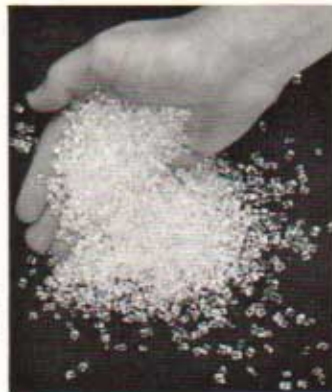
Rohm and Haas Plexiglas acrylic plastic molding pellets.
