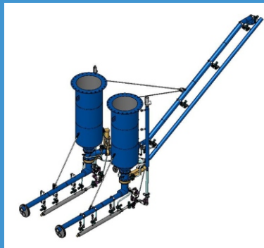
Stationary Dual SwallowTail™ Sea/Land Container Loading System with Bulk Bag Loader STINGER® Conveyor
