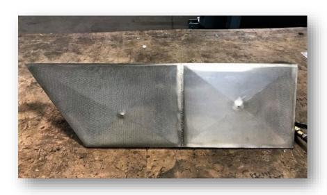
Special Transflow® Fludizing Pads were manufactured for the flat wall of a pyramid style hopper used in a bulk bag unloading station. The pads were an economical way to solve flow problems for this Pigment handling application. The pads were designed with two fluidization chambers. Each chamber was crimped to add strength to the Transflow® material. These pad's will utilize 3-5 PSIG compressed air.
