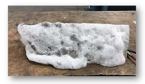
To demonstrate how the Transflow® pad distributes air uniformly over its surface, we pressurized the pad to 3 PSIG and sprayed a detergent solution on the pad. This shows how effective the Transflow® distributes the compressed air over the surface of the pad.
