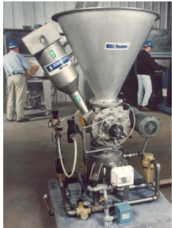
High Pressure rotary valve with transport vessel and air control piping
