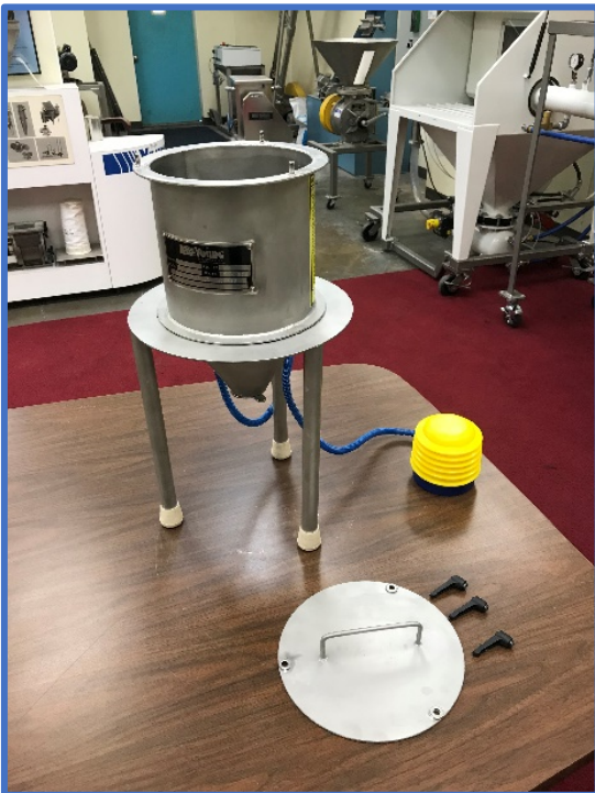
Transflow Hopper set up and ready for testing
