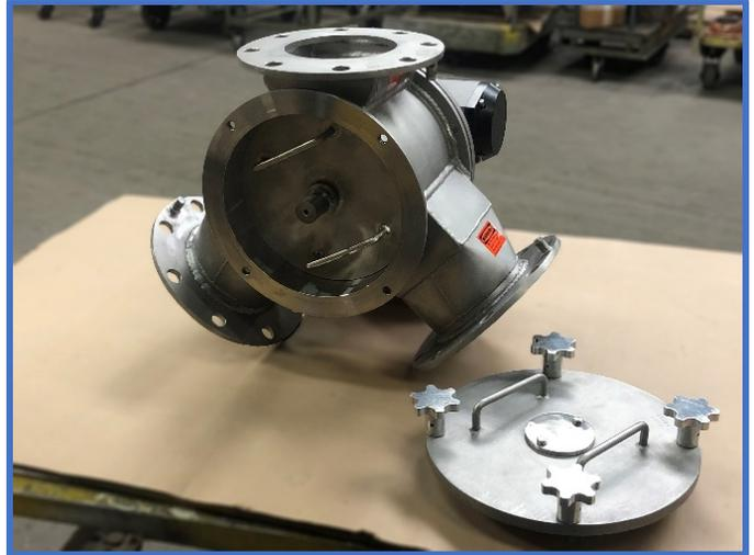
Cover Plate for Access to Remove the Rotor
