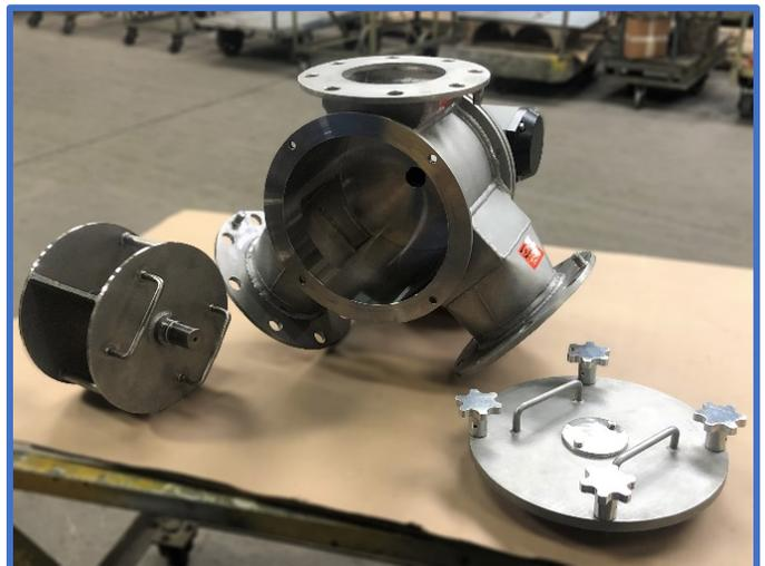
Rotor Removed with Complete Access to Interior
