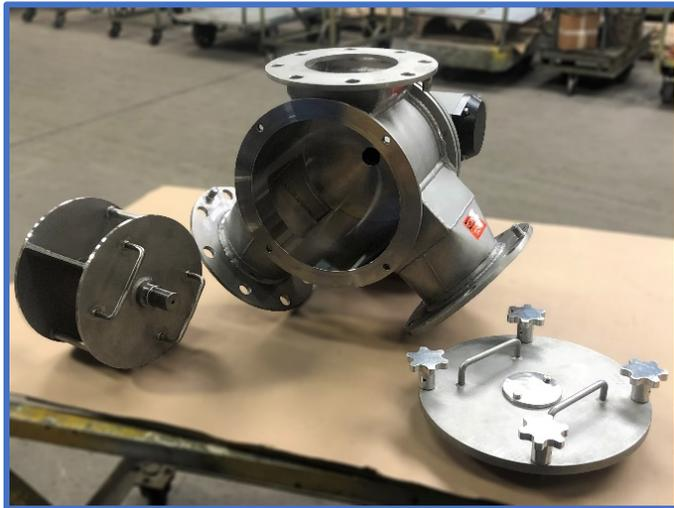
6" - Quick Clean Rotary Vane Diverter Valve
