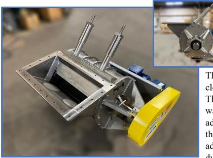
The Side Entry Rotary Valve was an easy choice for the metering requirement. The Side Entry allows for a maximum of 40% pocket fill and will not break or clip the beads. The 12" x 24" flange connection most closely matched the process vessel above. The requirement for variable flow control was solved by placing an external adjustment on to the inlet baffle to control the flow of beads into the rotor. Due to the added length of the valve, we supplied a dual external adjustment system.
