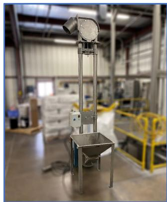
The Transvair Aero Mechanical Conveyor is manufactured in 304S/S and has a small inlet dump hopper. It has a grating (not shown in photo) that makes it easy for dumping paper bags or boxes of product into the hopper. The unit has a shaft mounted drive with TEFC motor and is complete with motor starter.
