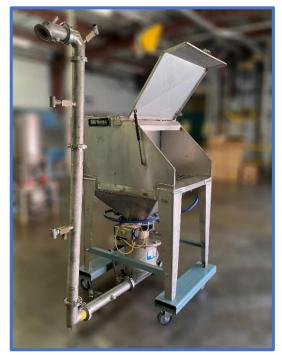
The Stinger Convey System conditions and fluidizes powders from inlet to discharge. The low velocity conveying system requires low pressure low volume compressed gas. The system is an excellent choice to convey fine powders from bags or bulk bags to process vessels.
