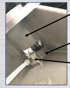
OUTBOARD MOUNTED BALL BEARINGS Open space between shaft seals and bearings
