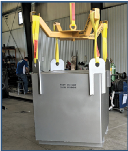
Load Testing Low Profile Lifting Bracket
