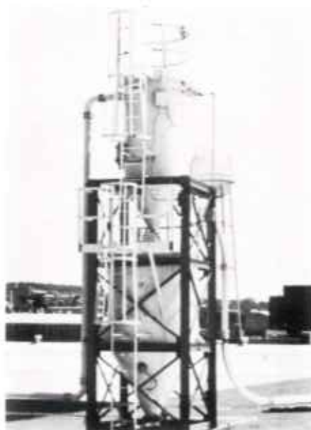
(left) Uni-Cage V/C Product Collector discharges into holding bin mounted below. Part of a TransVair Pneumatic System.
