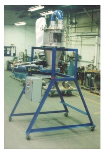
Receiving unit is self-contained and mounted on a frame for easy positioning over the customers' assembly machines. The units were completely assembled and tested before shipping to the plant.
