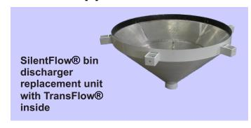
Discharger uses Trans-Flow® fluidizing media to condition the material to greatly reduce its internal friction angle. This allows the powder to freely discharge from cone openings as small as 4" in diameter.
