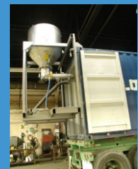
Portable SwallowTail™ Loader Mounted on Sea/Land Container
