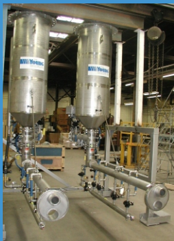
Stationary Dual SwallowTail™ Sea/Land Container Loading System with Bulk Bag Loader STINGER® Conveyor
