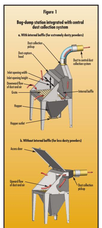
*velocity.* You can calculate this velocity using the method given in the following example, where the hood's inlet opening width (W) is 36 inches, its inlet opening height (H) is 24 inches, and the desired airflow draw is 150 fpm:
