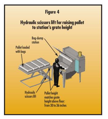
hood's inlet opening area not only handles the requirements of your pallet- or bag-lifting device, but easily handles the filled bag's size, the number of bags dumped per batch, and the number of batches per day or the batch operation's speed. A filled 50-pound bag is typically 30 to 36 inches long and 15 or 20 inches wide. To see how bag size, bag number, and batch speed affect the operator's work comfort and the hood's inlet opening area, consider the following examples:
