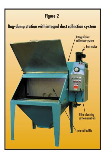
(typically from 40 to 60 psig) to be back-flushed into the filter interior for about 0.5 to 1 second. This back-flushed air passes through the media from the filter's clean side (interior) to the dirty side (exterior), forcing the dust to separate from the media and fall downward into the station's dust hopper. The pleated bag filter works well with most powders but may retain some cohesive powder between the pleats, ultimately reducing the usable filter surface area.
