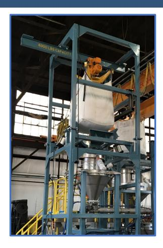
Young Industries lifting brackets comply with OSHA code 1926.251 and 1926.251 (a)(4). Each bracket is load tested with a weight equal to 125% of the lifting bracket rating. The photo on the left shows our Low-Profile Lifting Bracket with 10" offset being load tested with a 5000 lb. test weight. The lifting bracket will be used for a maximum lift of 4000 lbs.
