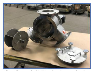
Rotor Removed with Complete Access to Interior
