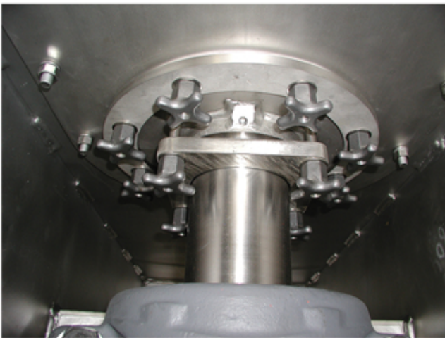
Sanitary Shaft Seal
