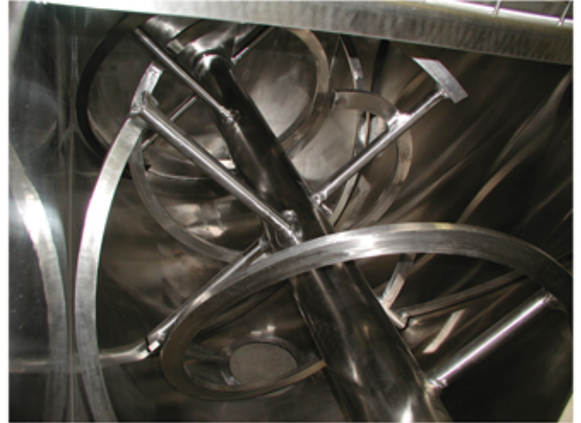
Multi-Pitch Agitator Sanitary Finish
